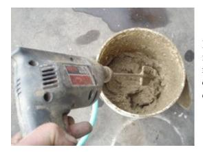
If you have access to electricity, a drill with a paint mixer attachment is a quick, satisfactory way to remove lumps in wet clay. Depending on the condition of the clay you may need to soak it several days.
